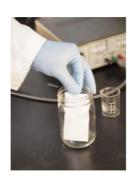
■ Place the test plate into the development container, it will lean at a slight angle with a coated side face up, and the edge with the samples toward the developing fluid . Make sure the bottom corners of the test plate are touching the side of the container. If the bottom of the test plate is not touching the side of the container, the developing solution may not be absorbed correctly. Put the lid on the developing container.
