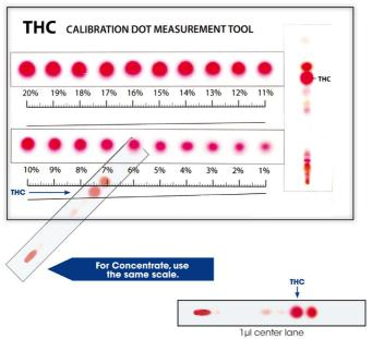
How to measure & calculate concentrates with Alpha-CAT 's THC calibration dot measurement tool
